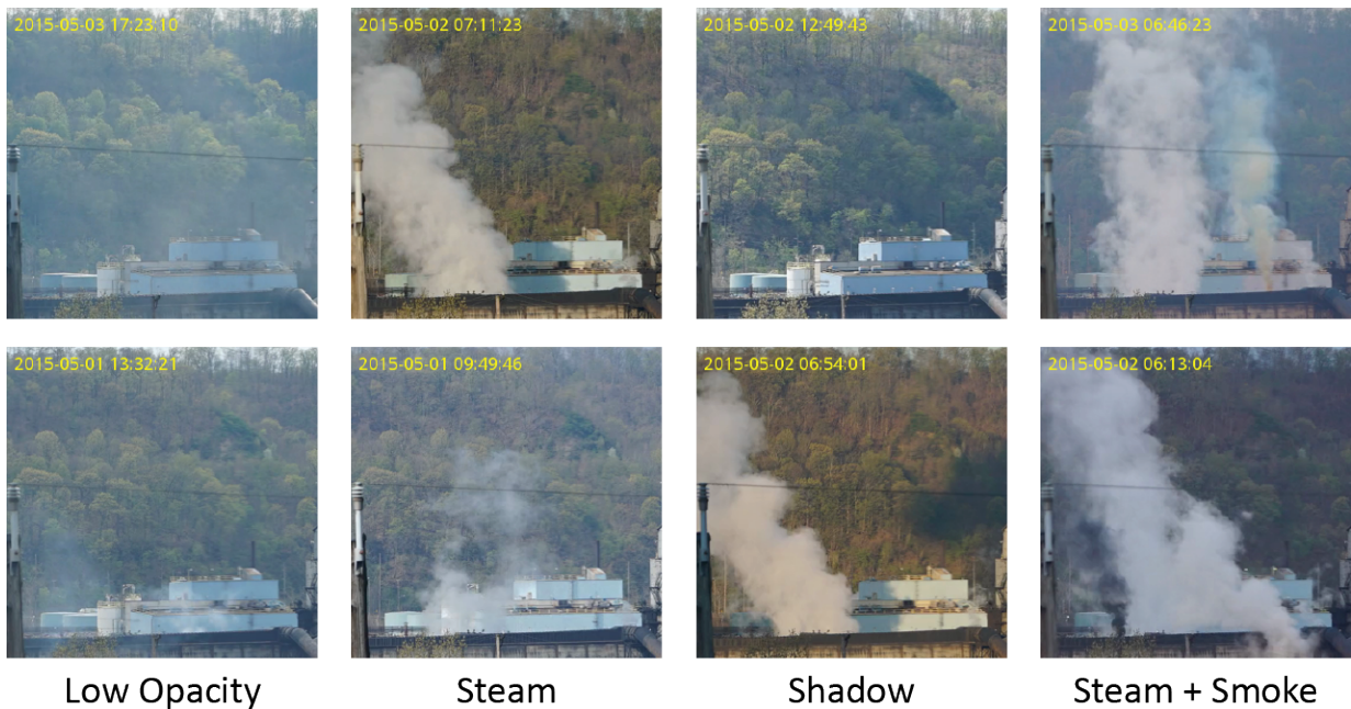
Figure 1.2: This figure shows steam, shadow, and the mixture of steam and smoke.
